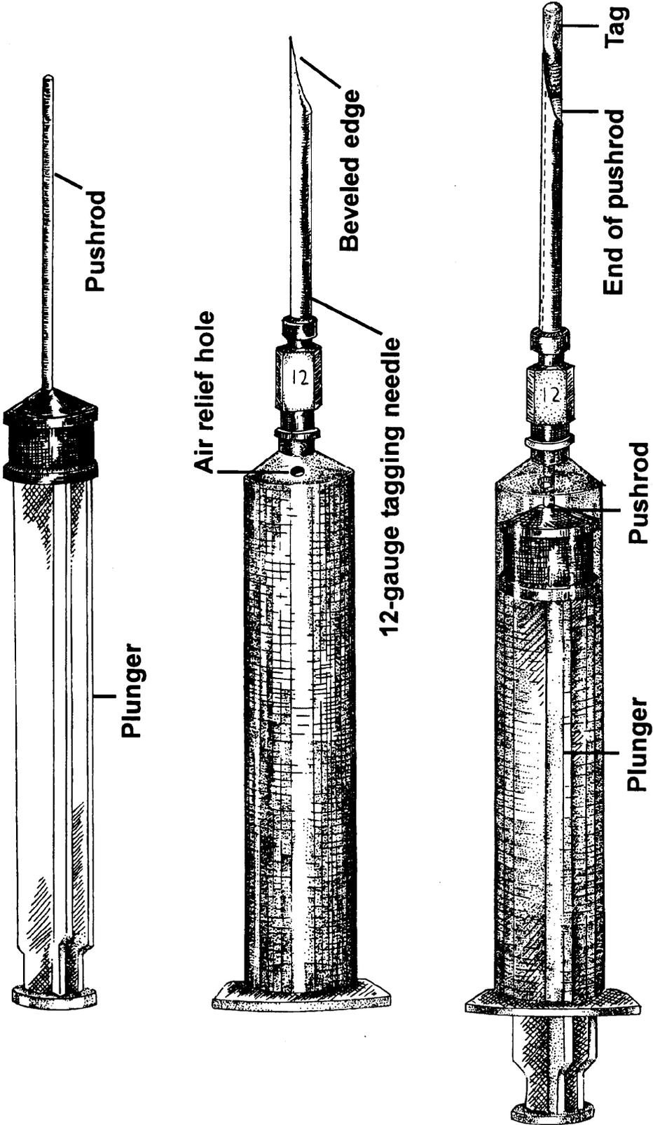
Figure 2. A spring-return PIT tag injector.
