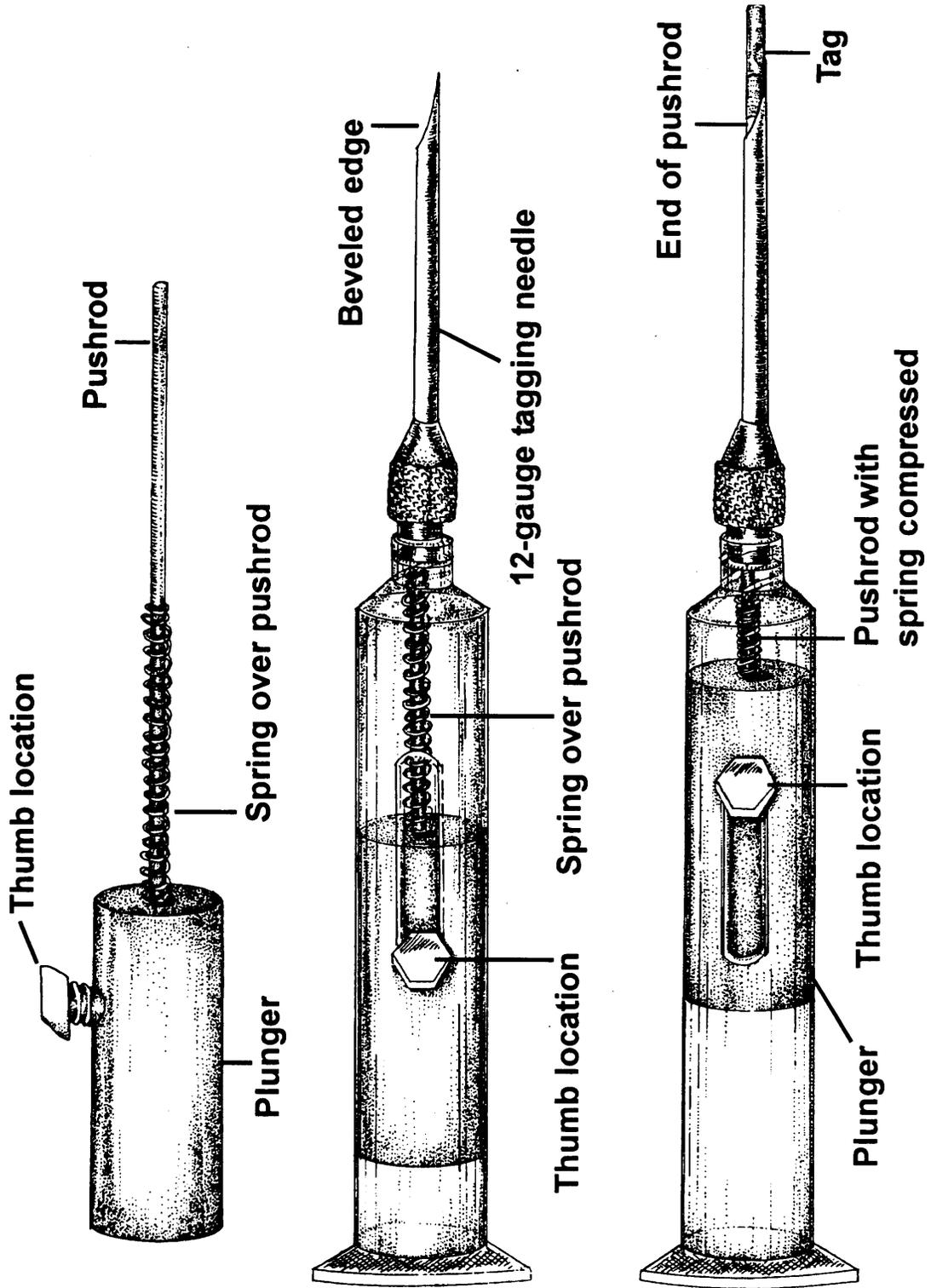
There are many possible variations to the hand held injector with the most elaborate incorporating thumb-operated plungers and springs in the barrel of the syringe to automatically retract the push rod (see Figure 2). The purpose of the spring is to keep the plunger retracted so it will not accidentally push the PIT tag out of the needle. To make this type of injector you will need:
